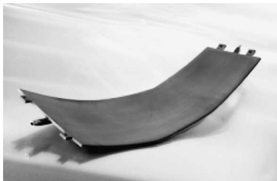
Fig. 1. Prototype of a full scale mock-up made by BUCO (Germany) and VPS-B 4 C covered by PLANSEE (Austria). The double wall panel made of stainless steel is Laser welded and embossed.
